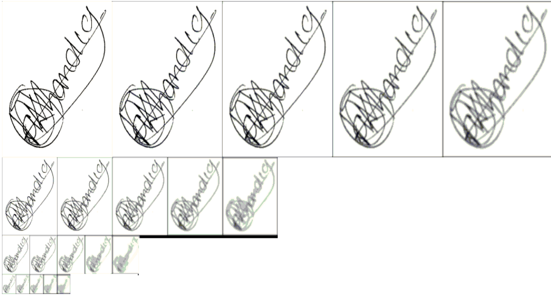
Figure 3.1: Example of space scale Gaussian images.
