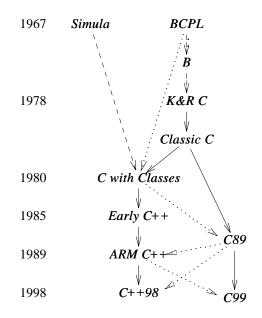
A solid line means a massive inheritance of features, a dashed line borrowing of major features, a dotted line borrowing of minor features.
