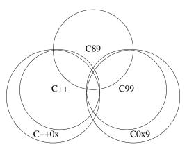
Each separate area of the diagram represents a set of incompatibilities that an implementer must address and that a programmer may have to be aware of.
