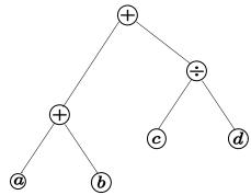
The top or root node in this case is the middle addition operation. The root node has two child nodes that can be considered as subtrees. The left child node of the root represents another addition operation for the a + b sum while the right child of the root node represents the division operation.
