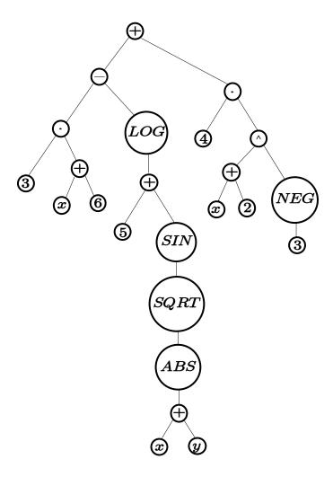
Again note that grouping symbols do not appear anywhere in the tree. Also note that only variables and constants appear as the bottom-most leaf nodes in the tree. All the interior tree nodes are either unary operators or binary operations.
