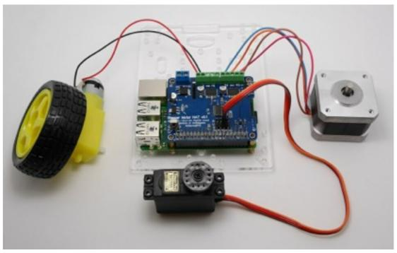
Let your robotic dreams come true with the new DC+Stepper Motor HAT. This Raspberry Pi addon is perfect for any motion project as it can drive up to 4 DC or 2 Stepper motors with full PWM speed control, It also adds the capability to control 4 Servos with perfect timing.
