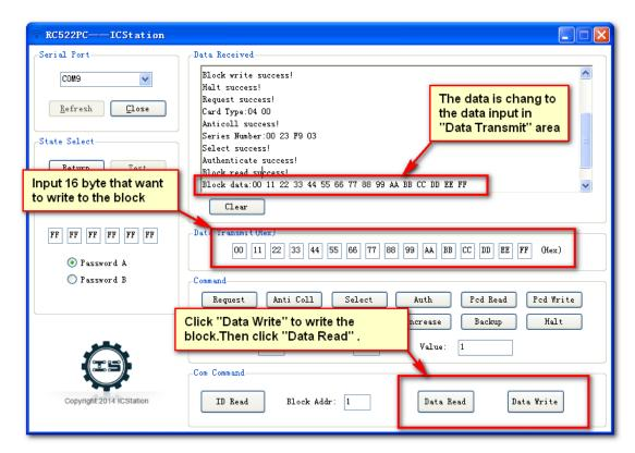
Command "Data Read" in "Com Command" area is equivalent to turn call "Request", "Anti Coll", "Select", "Auth", "Pcd Read", "Halt" in "Command" area.
