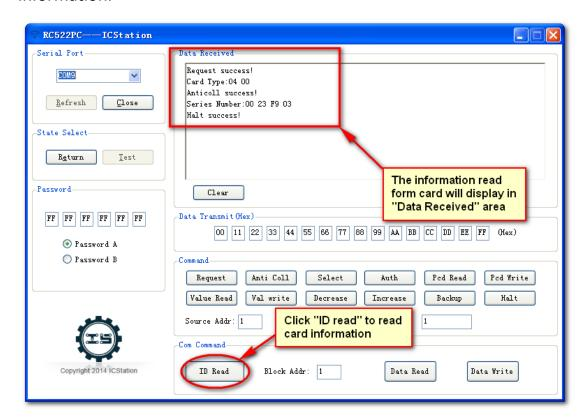
Command "ID read" in "Com Command" area is equivalent to turn call "Request","Anti Coll","Halt" in "Command" area.
