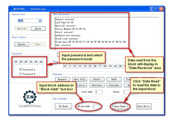
Command "Data Read" in "Com Command" area is equivalent to turn call "Request","Anti Coll","Select","Auth","Pcd Read","Halt" in "Command" area.Block address is range from 0 to 63.Card use password A "FF FF FF FF FF FF" in default.
